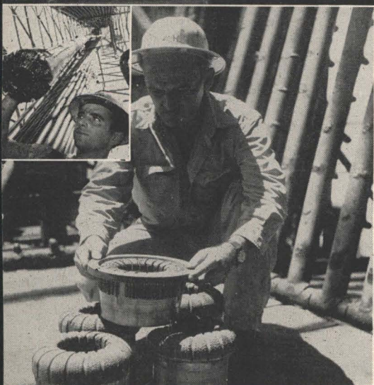
Driller Hyatt Harris checks diamond studded bit with ring gauge. Insert shows Rotary Helper Bill McLaughlin examining bit pulled from 20,246 ft. Penetration rates: 1 to 3 ft. per hr.
